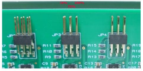
A link is fitted in one of the three positions as required.
